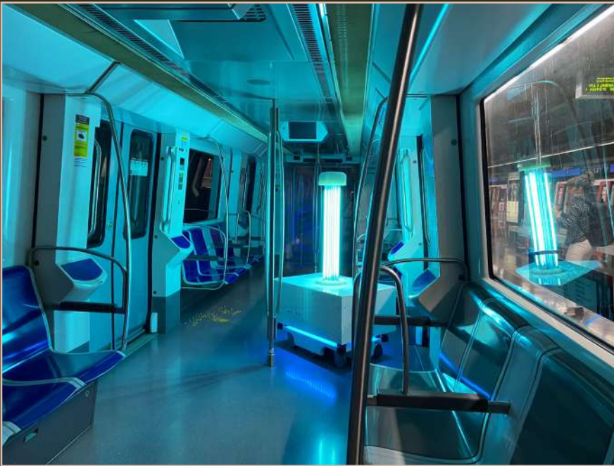
Fig. 6. Robot for disinfecting spaces MTS uvc, MTS uvc Team. © MTS tech
